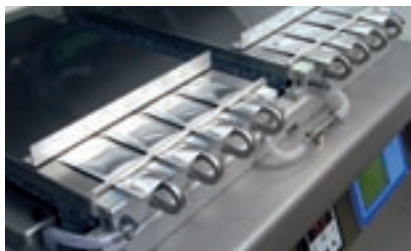
Gas injection into aluminium pouches via jets
